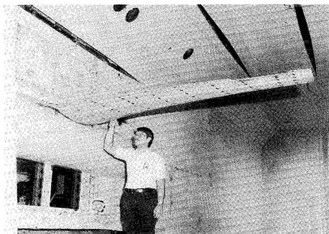
Fig. 1 Wing mounted in TDT test section.
